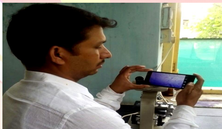
Figure 1: Holding the smart phone steady, the view below the microscope lens will show the photograph on the screen and an image can be captured by pressing right thumb
